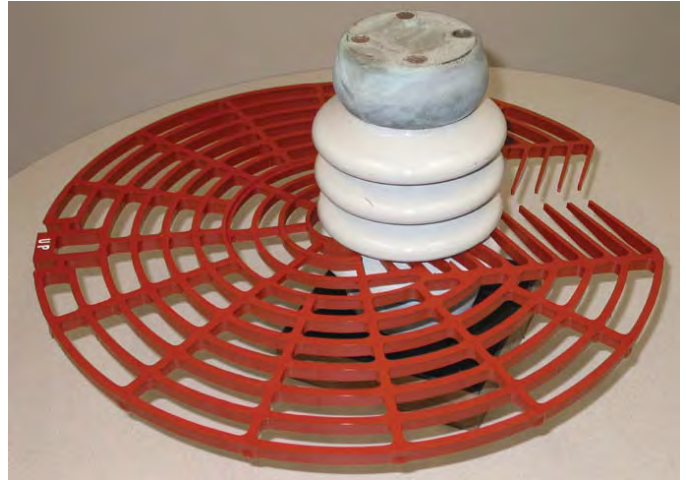
Figure 2: Improper Fit, Small Inner-Ring Diameter.
