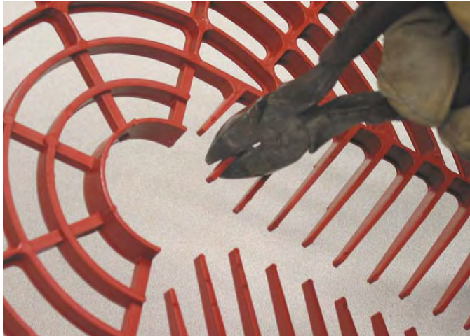
Figure 5: Trimming Flexible Fingers.
