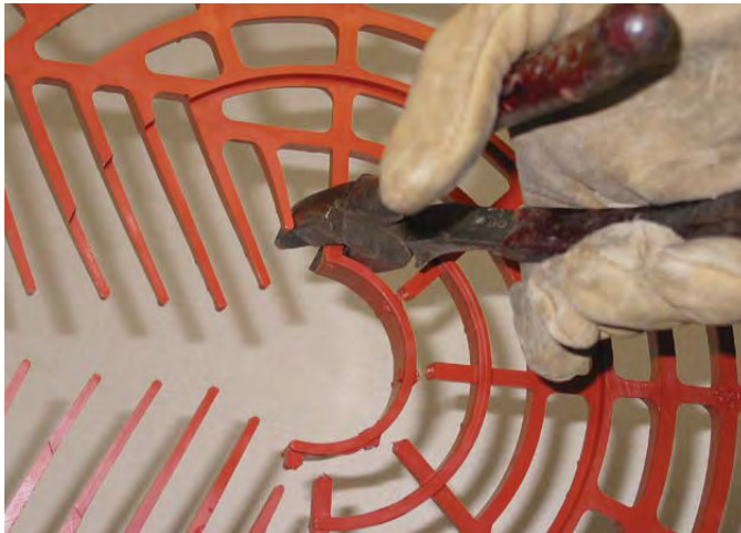
Figure 3: Adjusting Inner-Ring Diameter.
