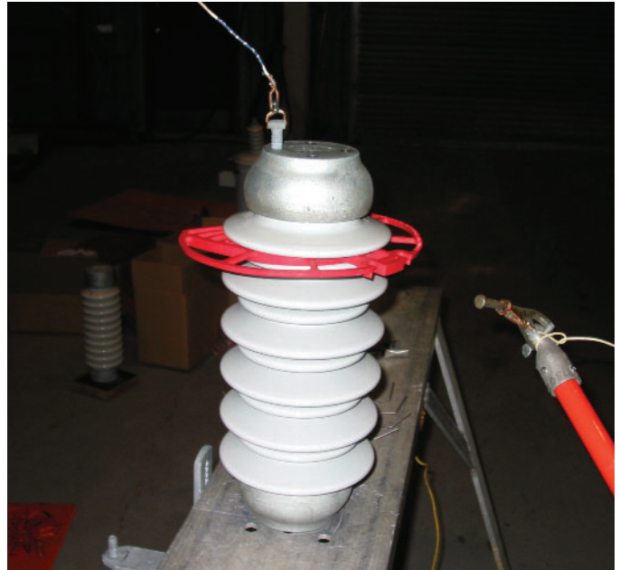
Figure 7: ZAPSHIELD Mounted Under 1st Major Diameter Skirt of a station post Insulator
