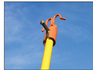
Slot to allow the prong of a disconnect (switch) stick to aid in installation and removal.
